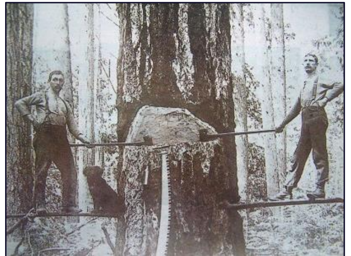
Photograph 14: Showing sawyers standing on planks inserted into notches cut into the tree. Crosscut saw leaning against the centre of the tree.
