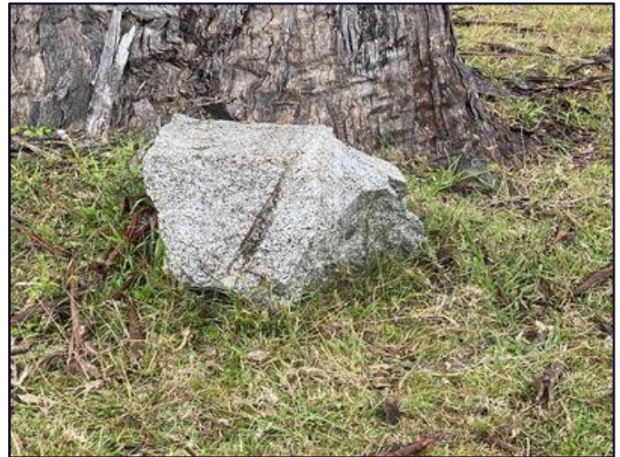
Photograph 10: Section of quarried granite with drill mark from quarrying. View to south-west.
